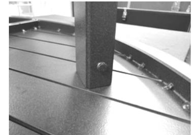
Fully tighten Locking Nuts that attach Table Support Brace (Optional), Leg Support Brace, and Leg (2 Locking Nuts, 4 places).
