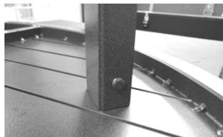
Fully tighten Locking Nuts that attach Table Support Brace (Optional), Leg Support Brace, and Leg (2 Locking Nuts, 4 places).
