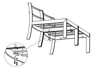
Fully Tighten bolts in both locations using a 7/16" combination wrench.
