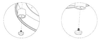
Install the glides by screwing them in to the bottom of the Fire Pit Riser. See diagrams below for both the Round Fire Pit Base and the Square Fire Pit Base.
