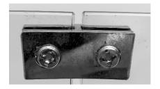
With the Upper Bracket Assembly Screw holes facing inward, slide the Upper Bracket over two joining Glass Panes. Lightly tighten the Set Screw with plastic nib to secure the Glass Panes with the Upper Bracket.
