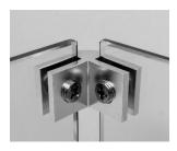
With the Upper Bracket Assembly Screw holes facing inward, slide the Upper Bracket over two joining Glass Panes. Lightly tighten the Set Screw with plastic nib to secure the Glass Panes with the Upper Bracket. DO NOT over tighten the screws. Over tightening may cause the glass to break.
