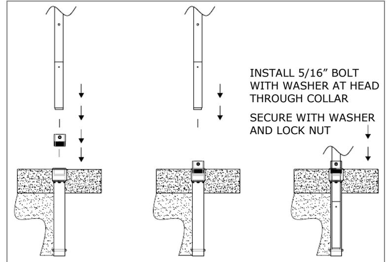
**WARNING:** The 5/16" bolt must not stick out from the lock nut and create a safety hazard.
