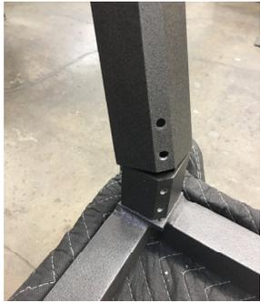
Attach leg with two bolts and two washers and fully tighten. Repeat for the remaining three legs.
