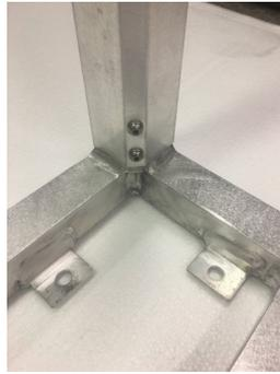
Check 8 bolts to ensure that all are fully tightened.
