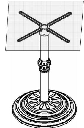
**CAUTION: Do not move the assembled table by lifting the Top. Two persons should move the table by lifting the Spider Support arms.**
