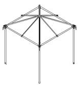
WARNING: Screws and Locking Nuts must be fully tightened to secure Poles to Corner Bracket Assemblies. Failure to do so may cause Corner Poles to separate from Corner Bracket Assemblies and result in injury to persons or damage to property.
