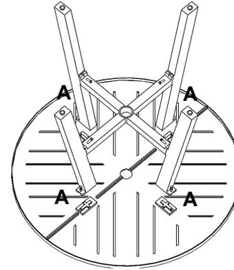
Loosely attach each leg with One **(A)** bolt and two washers. Do not fully tighten until all four legs are attached.
