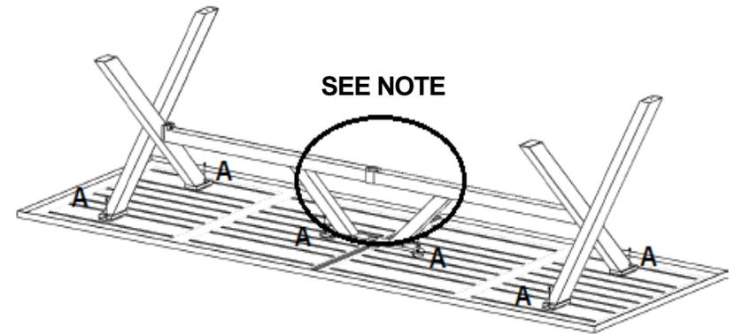
Loosely attach each leg with One **(A)** bolt and two washers. Do not fully tighten until all four legs are attached.
